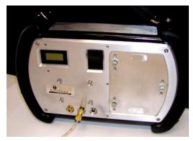
To use the TRACER with vacuum, connect the instrument's vacuum line and the pump vacuum line. Be sure to connect with relief port on instrument side (not pump side).
